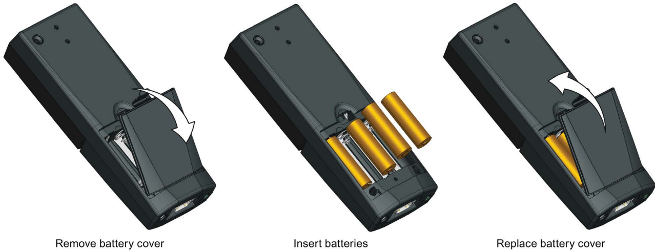
Figure 7-4 Installing batteries for handheld kit
