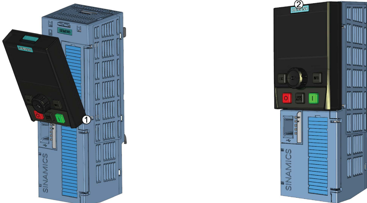
Figure 3-1 Fitting the IOP to the Control Unit
